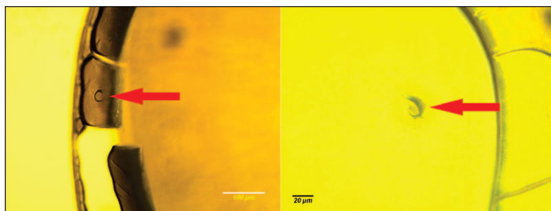
Figure 2. Light microscopy photographs display microvortex profiles (arrows) in nanocrystalline igloos grown under identical conditions on different hydrophobic surfaces: Polystyrene (left) and nanocrystalline diamond (right). As a general tendency, microtornadoes develop more frequently on polystyrene than on nanocrystalline diamond.
